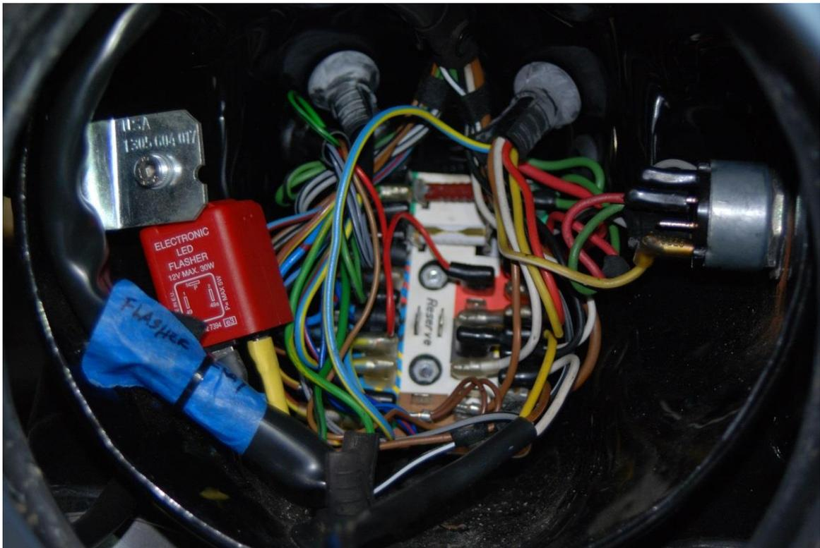
The flasher relay and connections need to be out of the way of the rear of the headlight assembly.
