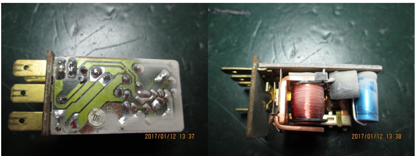
Remove the outer shell, and inspect interior. These photos show lots of grey (shorting) dust.
