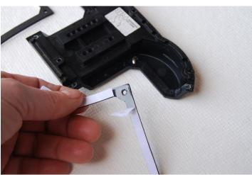
Tweezers can help push the square piece down evenly over the machine screw, to stick it on flat and square to the right angle edges as shown.
