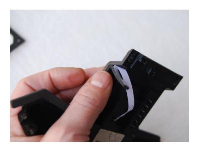
Now peel a little more of the backing off, enough to uncover the adhesive for the corner. Bend the gasket and press the corner in tight to the Rear Cover. Remember to keep the edge of the gasket aligned with the outside edge of the Rear Cover.
