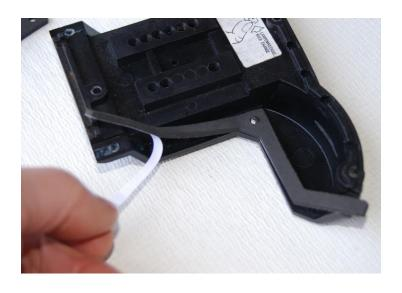
**3.** Partially remove the backing on the longer straight foam strip. Leave the backing on the section over the bend for now. (see photo) The adhesive on these strips is quite good, and it will not peel off if you stick it on in the wrong location.
