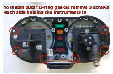
I. REMOVE YOUR GAUGES. After you have removed your instrument pod from the bike, and gotten to the part where you've removed your oem light board, it will look like this. Now remove the 3 screws on each side that hold the speedo and tach in. Set the instruments carefully to the side, on their sides (not their face as it will damage the indicator needle). Remove the old Oring in the slot around the perimeter.
