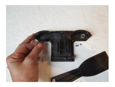
I. REMOVE YOUR EXISTING OLD GASKET. I've done 3 of these, and they were all very easy to remove. I could just peel the old one right off, then rub the remaining cement off with my thumb. If you have to- use a *plastic* scraper- so you don't damage the Rear Cover. Then wipe the gasket area with lacquer thinner to remove all traces of old adhesive and oils.
