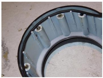
**3**. Work your way around, holding the O-ring on the shelf with your thumb, and tucking it in behind the pins. Do not pry against the pins- they WILL break off. I use a small slot blade screw driver. Do not use anything sharp as it will puncture or cut the soft O-ring material.
