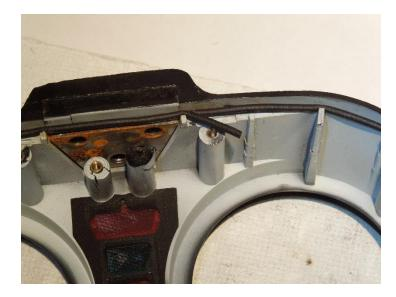
4. When you get to the end, there will be about a half inch overlap. Trim it with a scissors if it's too long. Finish with the end to the inside of the pod to hold the starting end of the O-ring in place.
