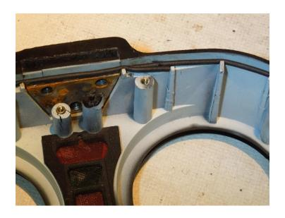
**5.** Finish with a TINY dab of gel super glue. I put some super glue on a piece of scrap paper, then use a toothpick to apply it to the side of the Oring and tack it to the other end. DO NOT glue your finger OR the Oring to the case.
