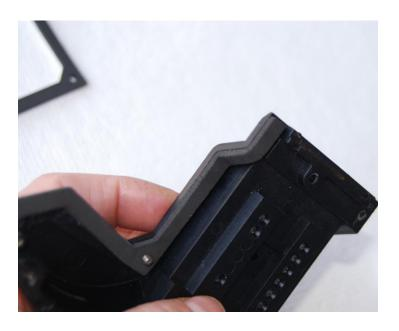
Finally you can peel off the remainder of the backing and finish pressing the new seal onto the edge of the Rear Cover.
