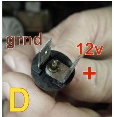
You do not need to disconnect the wires to the socket, but you **DO** need to check that they are connected for the correct polarity! The grey wire is the 12v in and should be connected to the 12v terminal. See photo **D** on the right. The brown is the ground. If you do not have the wire connections correct the led bulb will not light up.
