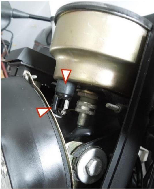
Photo left: speedo light socket. Just pull down to remove.
